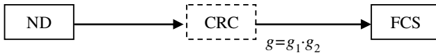
Fig. 2. CRC with a generator polynomial that is a product of two polynomials
